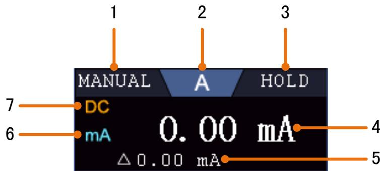
Figure 6-3 Multimeter Information Window
