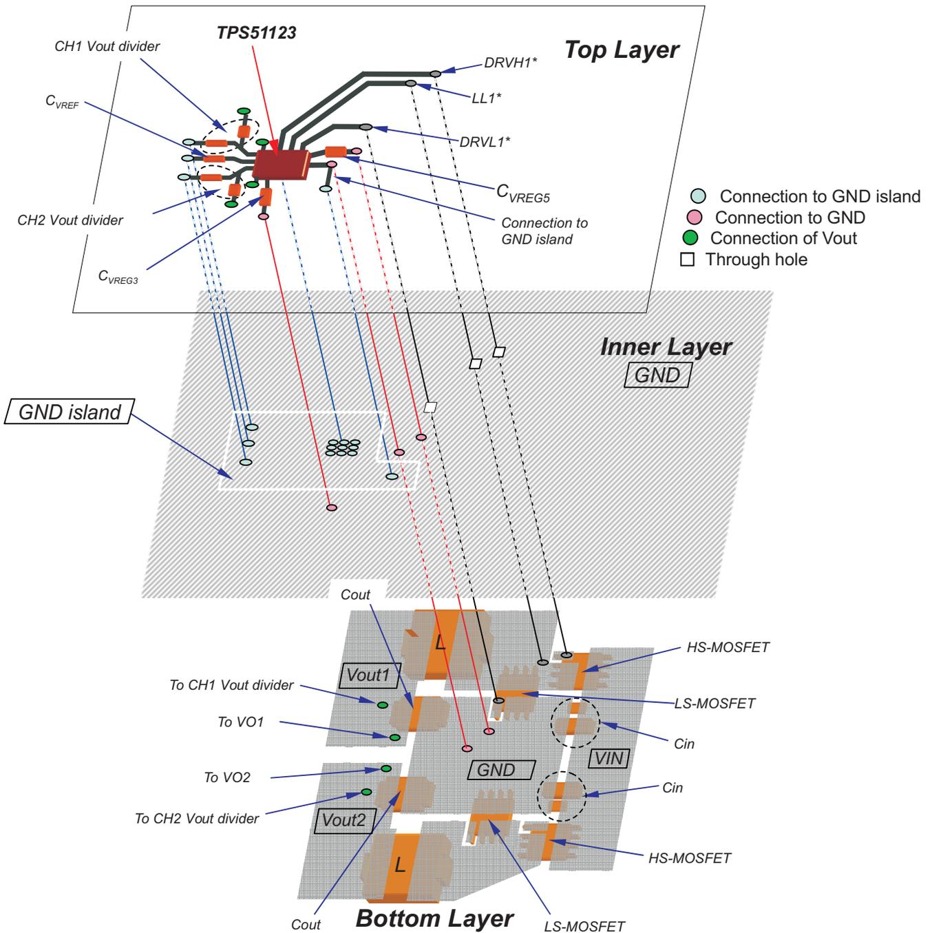
Figure 38. PCB Layout
