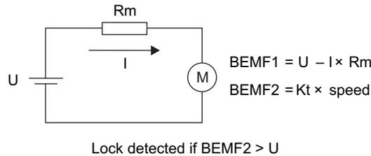
**Figure 29. Lock Detection 1**
