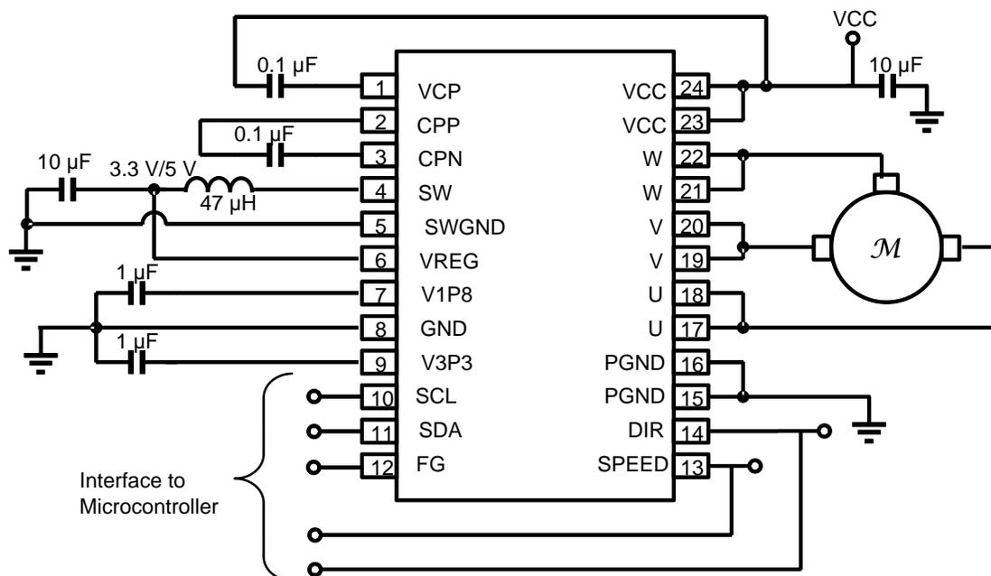
**Figure 40. Typical Application Schematic**
