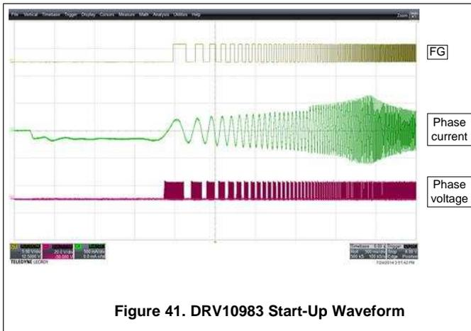
**Figure 41. DRV10983 Start-Up Waveform**
