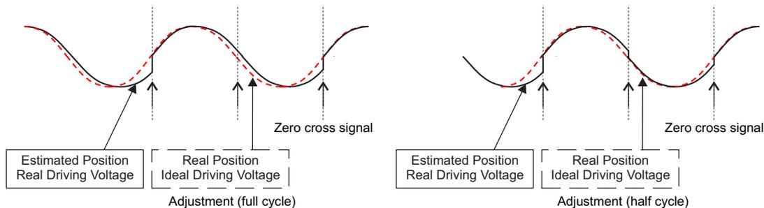
Figure 20. Closed Loop Control Commutation Adjustment Mode
