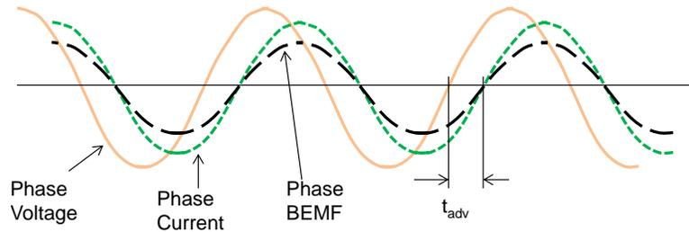
Figure 25. Advance Time ( $t_{adv}$ ) Definition
