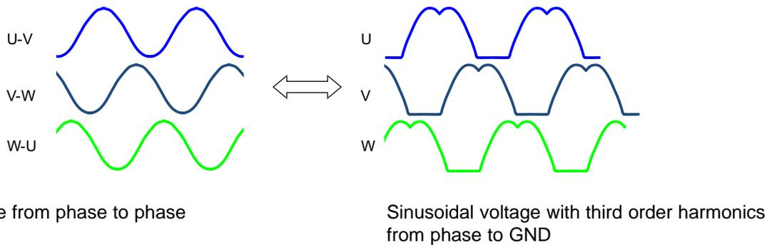
Figure 7. Representing Sinusoidal Voltages With Third-Order Harmonic Output
