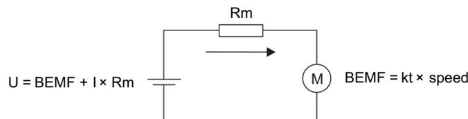
Figure 18. Motor Start-Up Current
