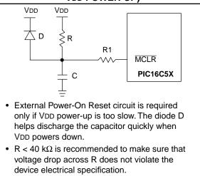
• R1 =  $100\Omega$  to 1 k $\Omega$  will limit any current flowing into  $\overline{MCLR}$  from external capacitor C in the event of  $\overline{MCLR}$  pin breakdown due to Electrostatic Discharge (ESD) or Electrical Overstress (EOS).
