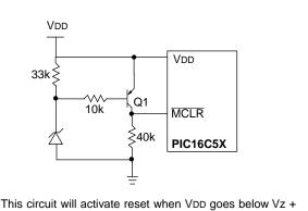
This circuit will activate reset when VDD goes below Vz + 0.7V (where Vz = Zener voltage).
