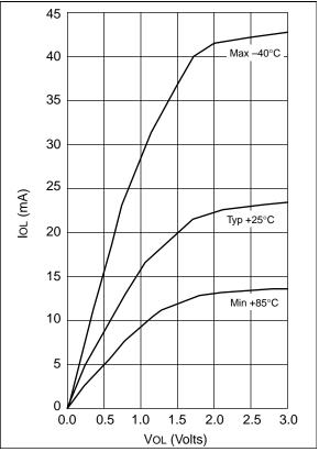
FIGURE 20-18: IOL vs. VOL, VDD = 5 V
