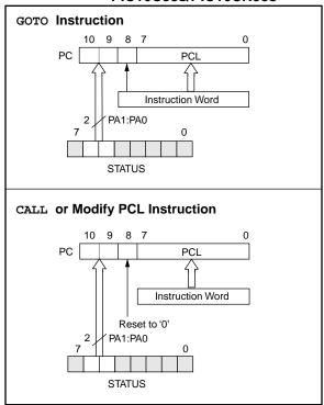
For the RETLW instruction, the PC is loaded with the Top Of Stack (TOS) contents. All of the devices covered in this data sheet have a two-level stack. The stack has the same bit width as the device PC. 4.5.1 PAGING CONSIDERATIONS – PIC16C56s/CR56s, PIC16C57s/CR57s AND PIC16C58s/CR58s
