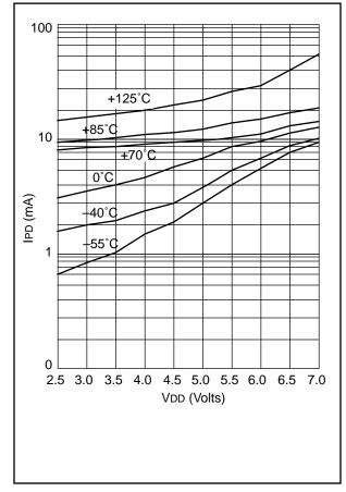
FIGURE 12-7: TYPICAL IPD vs. VDD, WATCHDOG ENABLED
