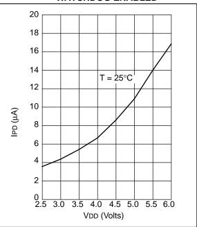
FIGURE 12-8: MAXIMUM IPD vs. VDD, WATCHDOG ENABLED
