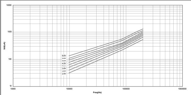
FIGURE 18-12: TYPICAL IDD vs. FREQUENCY (WDT DIS, RC MODE @ 100 PF, 25°C)
