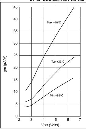
FIGURE 12-17: TRANSCONDUCTANCE (gm) OF LP OSCILLATOR vs. VDD
