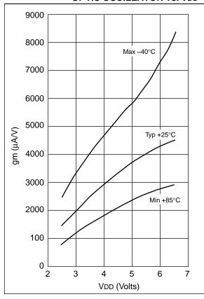
FIGURE 18-17: TRANSCONDUCTANCE (gm) OF HS OSCILLATOR vs. VDD
