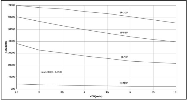
FIGURE 18-4: TYPICAL RC OSCILLATOR FREQUENCY vs. VDD, CEXT = 300 PF
