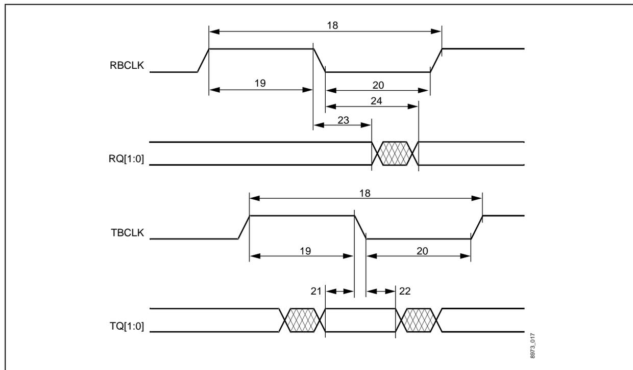
**Figure 5-4. Channel Unit Interface Timing, Parallel Slave Mode**
