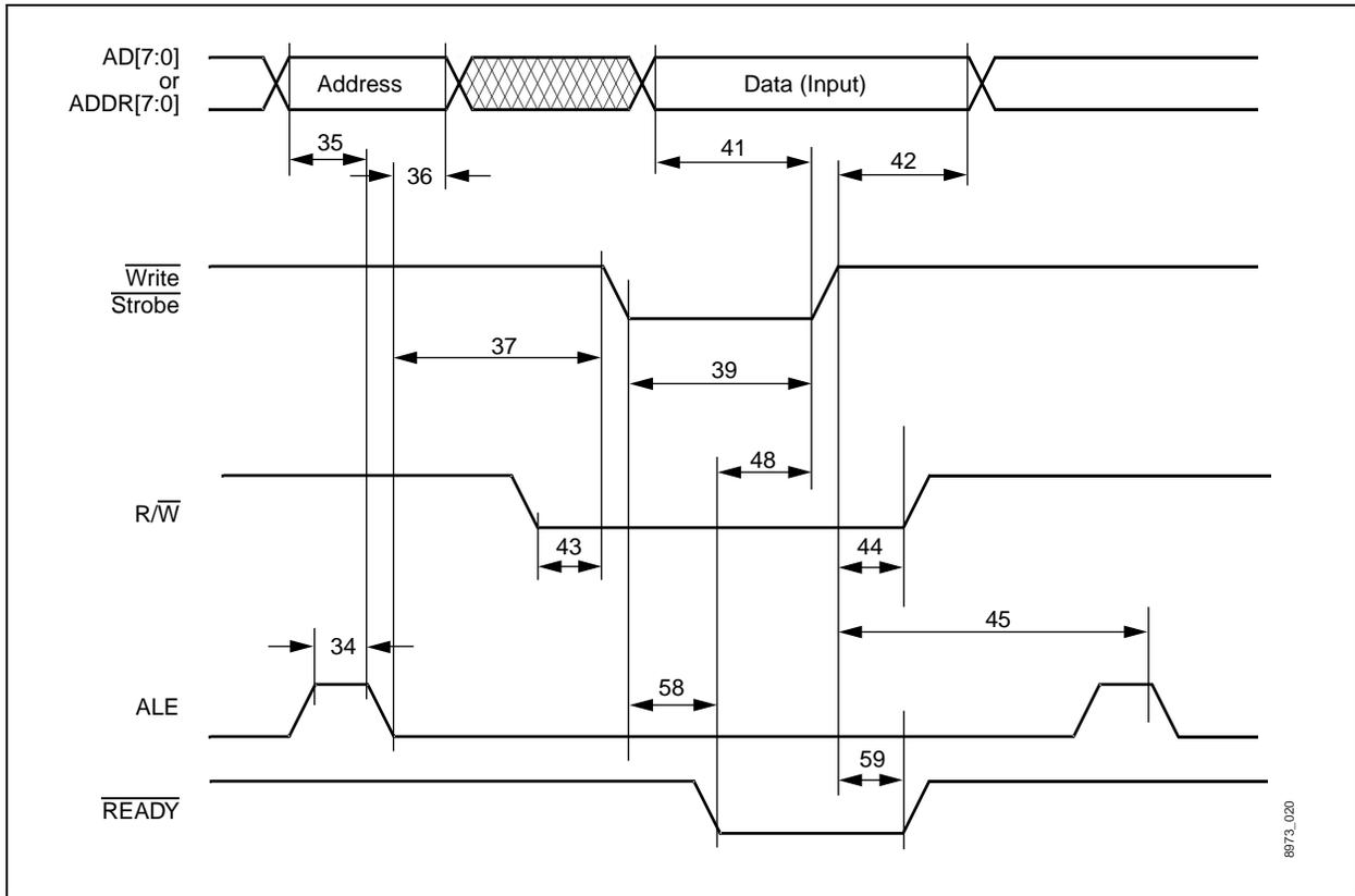
Figure 5-8. MCI Read Timing, Intel Mode ( $\overline{MOTEL} = 0$ )
