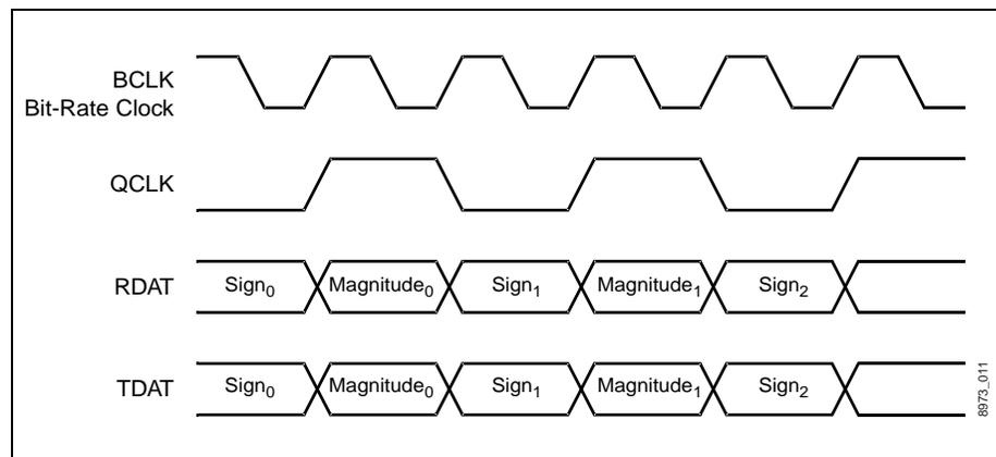
In parallel master mode, the sign and magnitude receive data is output through RQ[1] and RQ[0], respectively, on the rising edge of QCLK. The quaternary transmit data is sampled on the falling edge of QCLK. This clock and data relationship is illustrated in [Figure 2-7](#).
