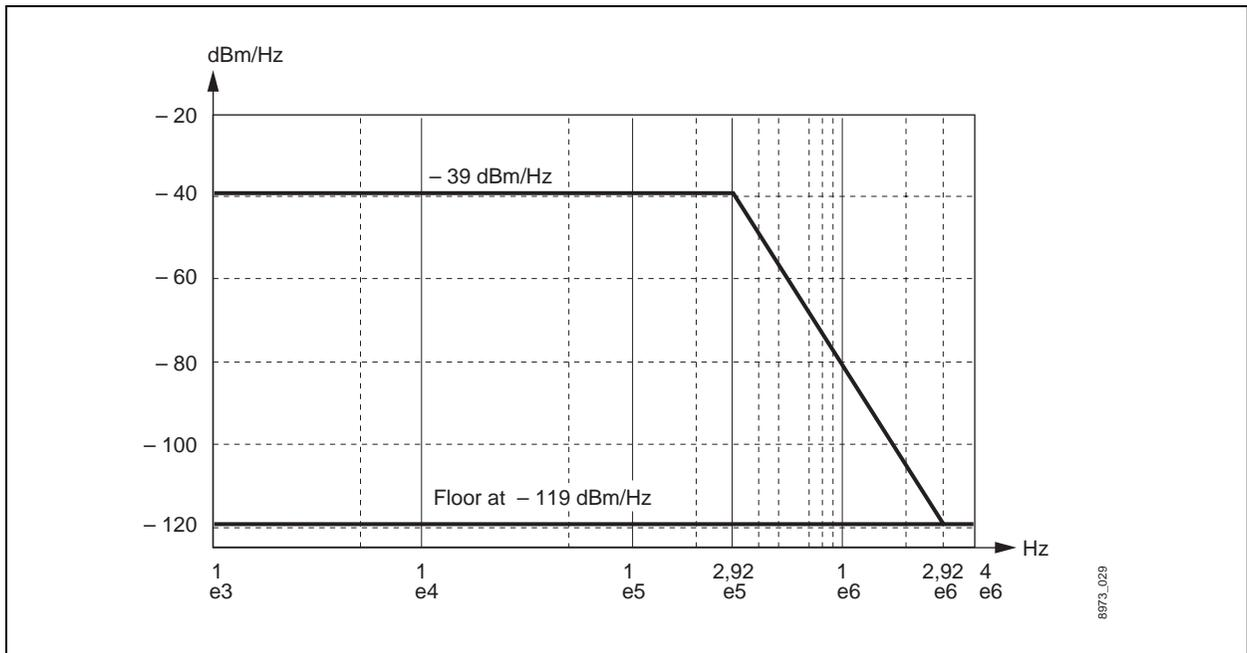
Figure 5-17. Upper Bound of the Average PSD of a 1160 kbaud System (Source ETSI TS 101 135 Formerly ETR 152)
