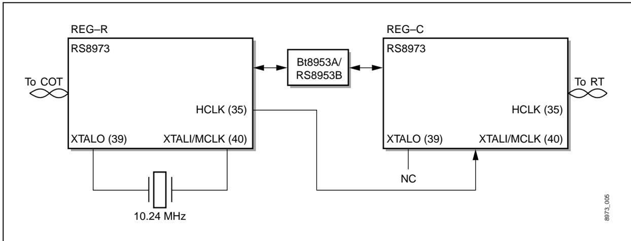
HCLK on REG-R is configured to run at 16 times the symbol rate, which is the power-on default.
