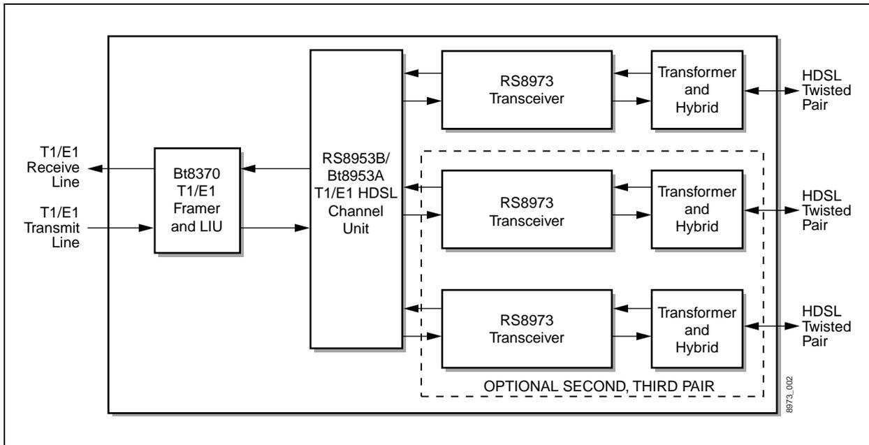
The RS8973 comprises five major functions: a transmit section, a receive section, a timing recovery and clock interface, a microcomputer interface, and a test and diagnostic interface. Figure 1-2 details the connections within and between each of these functional blocks.
