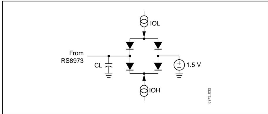
Figure 5-20. Open-Drain Output Load ( $\overline{IRQ}$ )
