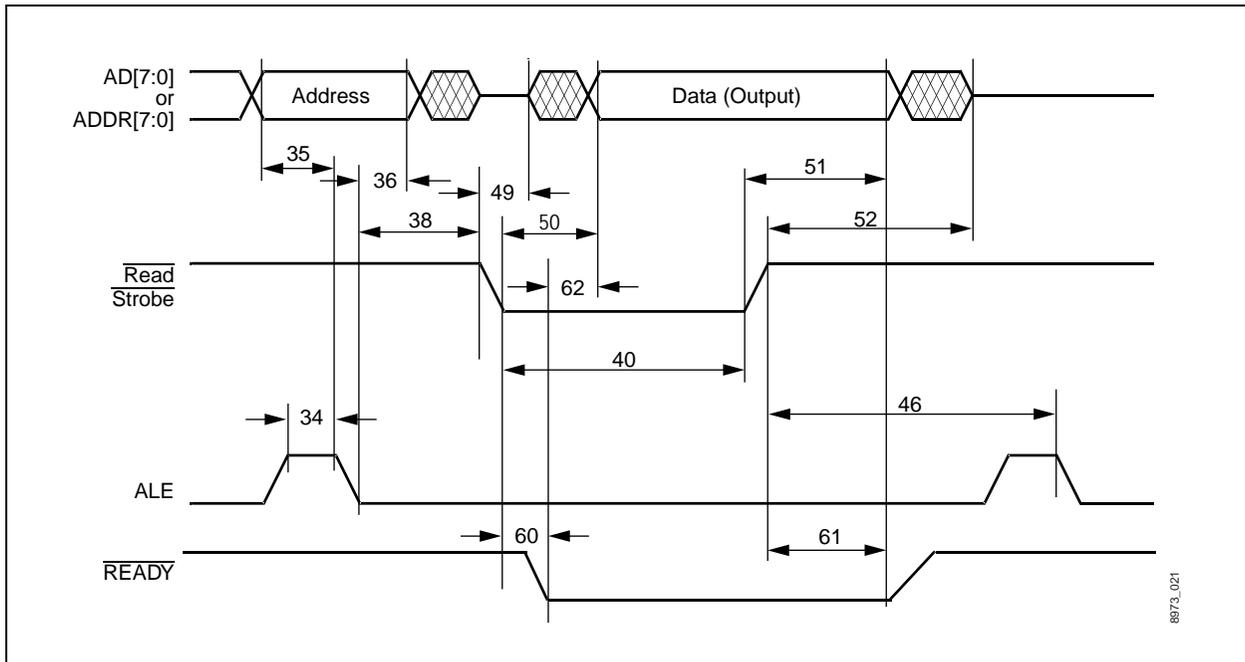
Figure 5-9. MCI Read Timing, Motorola Mode ( $\overline{MOTEL} = 1$ )
