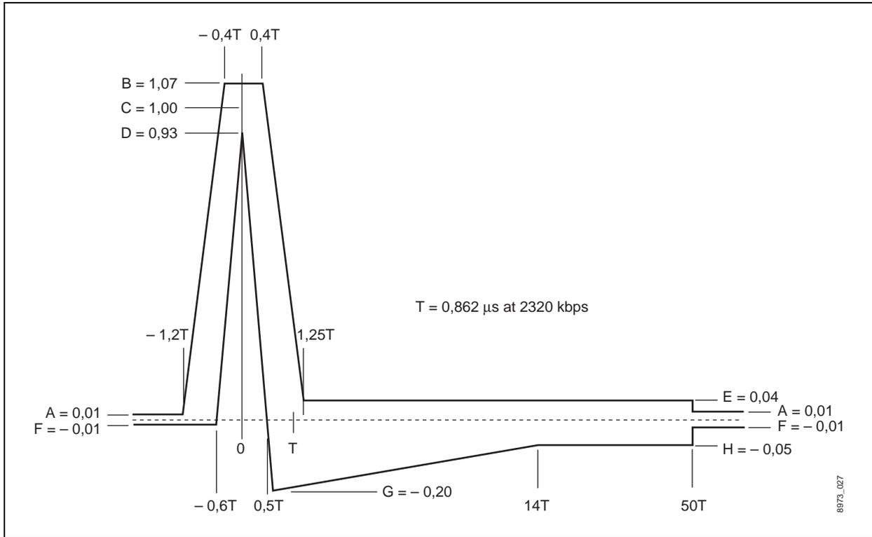
Table 5-20. Transmit Pulse Template for One-Pair Systems (Source ETSI TS 101 135 Formerly ETR 152)
