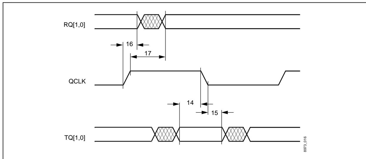
Table 5-9. Channel Unit Interface Timing Requirements, Parallel Slave Mode
