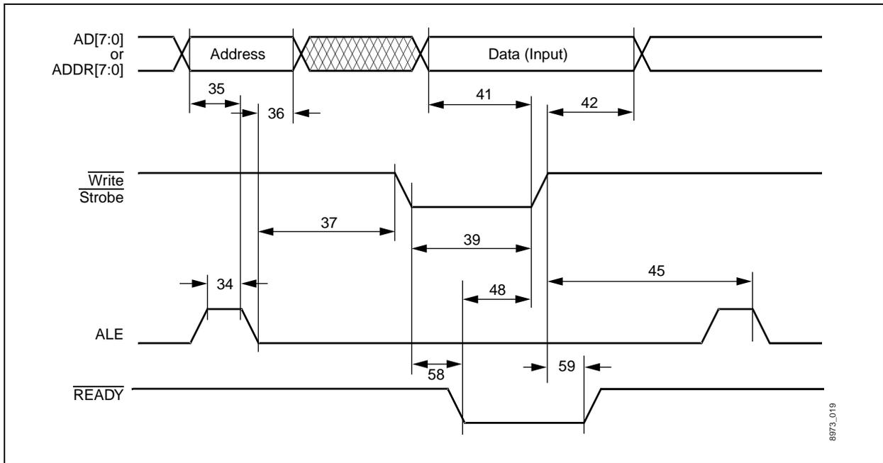
Figure 5-7. MCI Write Timing, Motorola Mode ( $\overline{MOTEL} = 1$ )
