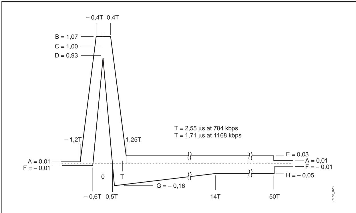
Table 5-19. Transmit Pulse Template for Two- and Three-Pair Systems (Source ETSI TS 101 135 Formerly ETR 152)
