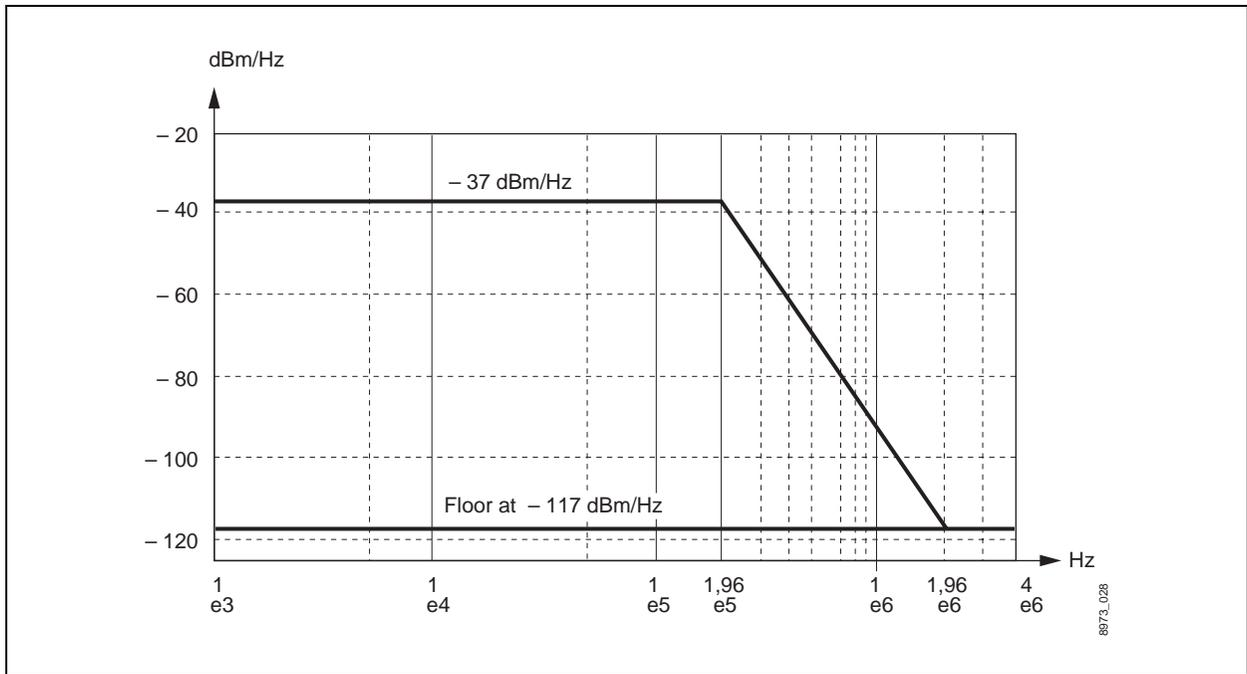
Figure 5-16. Upper Bound of the Average PSD of a 584 kbaud System (Source ETSI TS 101 135 Formerly ETR 152)
