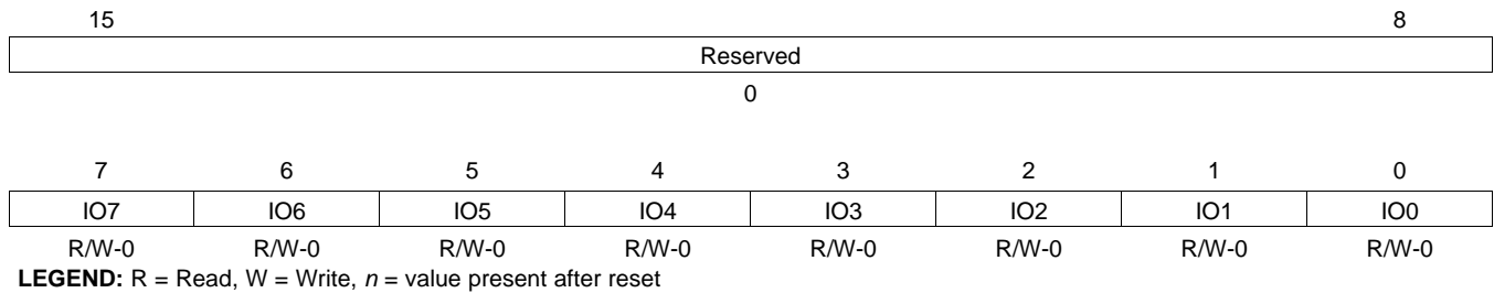
Figure 3-21. General-Purpose I/O Status Register (GPIOSR) [MMR Address 003Dh]
