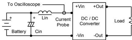
**Peak-to-Peak Output Noise Measurement Test**
