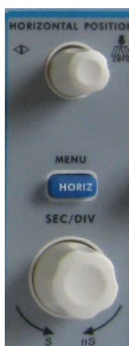
Fig. 4-13 Horizontal Control Zone
