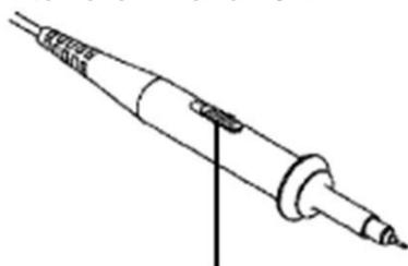
Figure: Attenuation Switch
