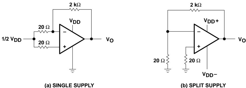
Figure 2. Noise-Test Circuit
