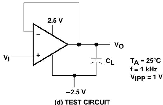
Figure 41. Effect of Capacitive Loads and Test Circuit
