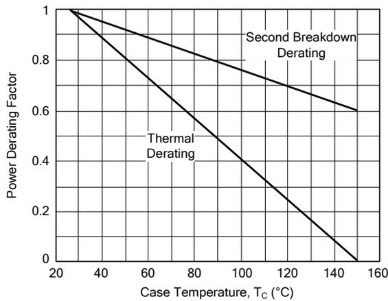
There are two limitations on the power handling ability of a transistor: average junction temperature and second breakdown. Safe operating area curves indicate  $I_C - V_{CE}$  limits of the transistor that must be observed for reliable operation; i.e., the transistor must not be subjected to greater dissipation than the curves indicate.
