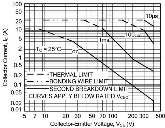
Fig. 2 Reverse Bias Switching Safe Operating Area
