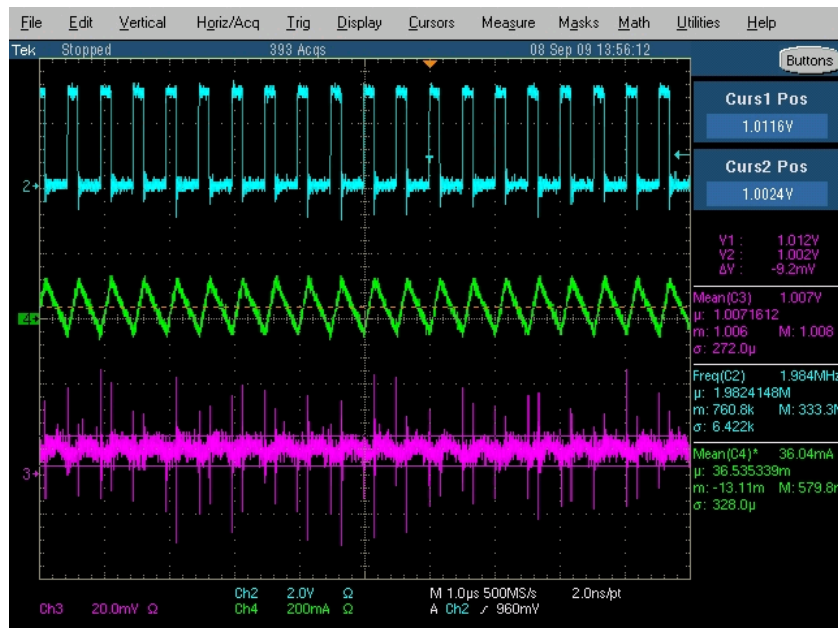
Figure 19. L=GTSD32P-2R2M, C=Ceramic 4.7μF 0805 X5R TDK (Ripple 9.2mV)
