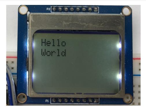
Notice the second line of text starts at Y position 10, this moves it down the display 10 pixels so it's below the first line of text. The font used by the text function is 8 pixels tall so a size of 10 gives a bit of room between the lines.
