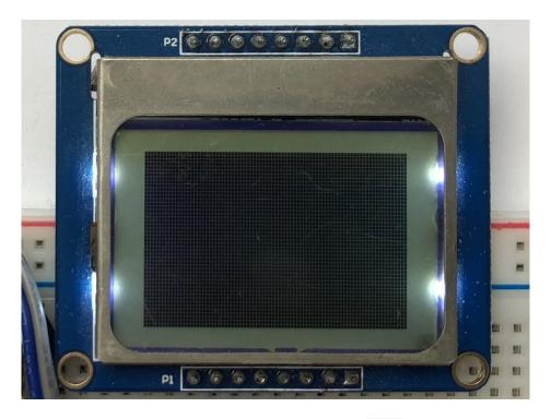
Notice the fill function doesn't actually change the display. You must call show after making drawing commands to send the updated pixel data to the display!
