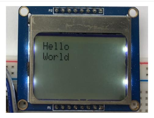
That's all there is to drawing on the Nokia 5110/3310 LCD display with CircuitPython! The drawing functions are basic but provide building blocks for more advanced usage. For example you can display text with sensor readings or other state, or even program a simple game like pong!
