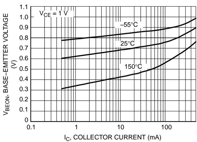
Figure 4. Base-Emitter Voltage
