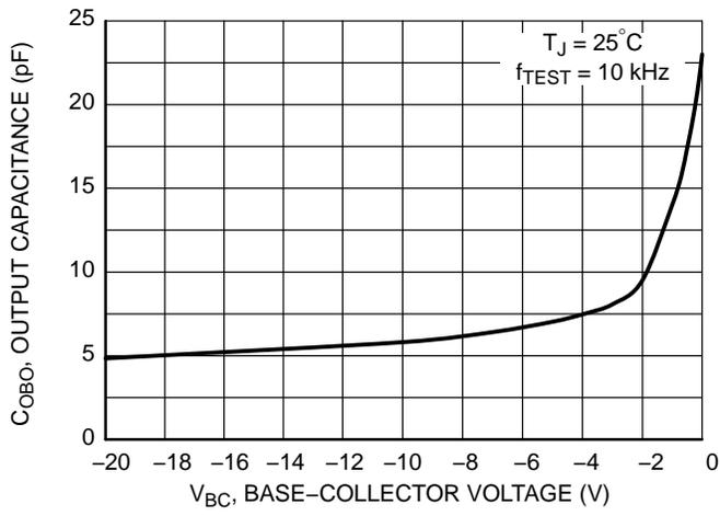
Figure 7. Output Capacitance
