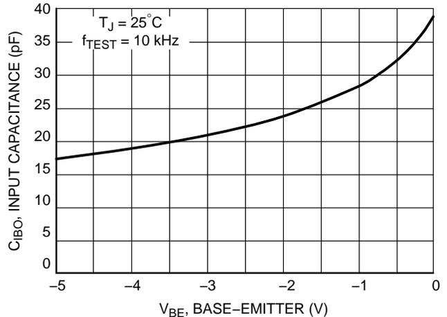
Figure 6. Input Capacitance
