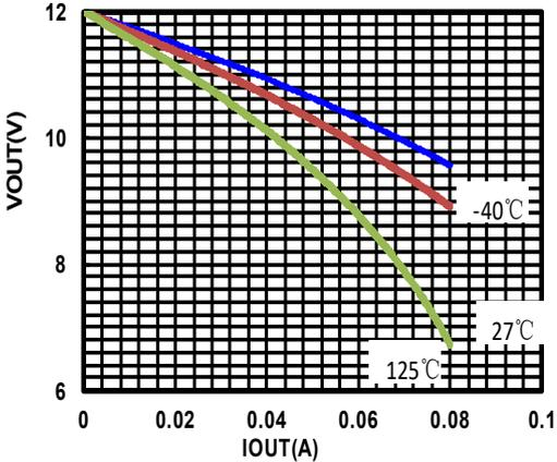
Negative Output Swing vs. Load Current
