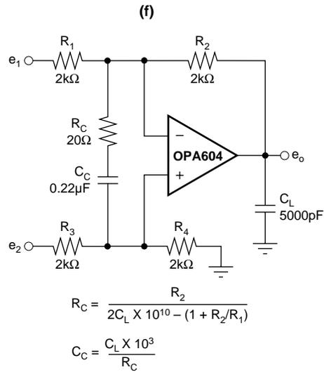
NOTE: Design equations and component values are approximate. User adjustment is required for optimum performance.
