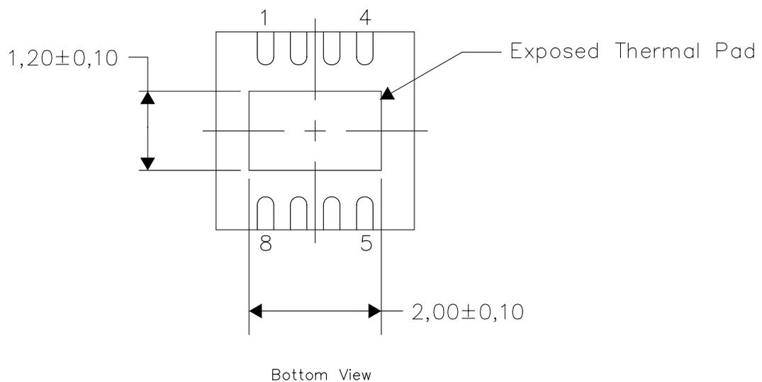
NOTE: All linear dimensions are in millimeters
